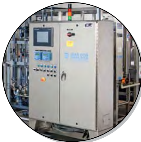
NEMA 4X control panel
